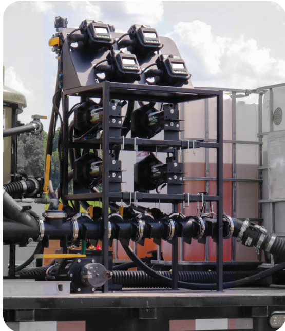
Direct inject herbicides into the carrier flow.
